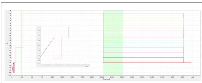
Fig. 3: Voltage protocol with ramp and prepulse for reversal potential investigations with leak corrections.
