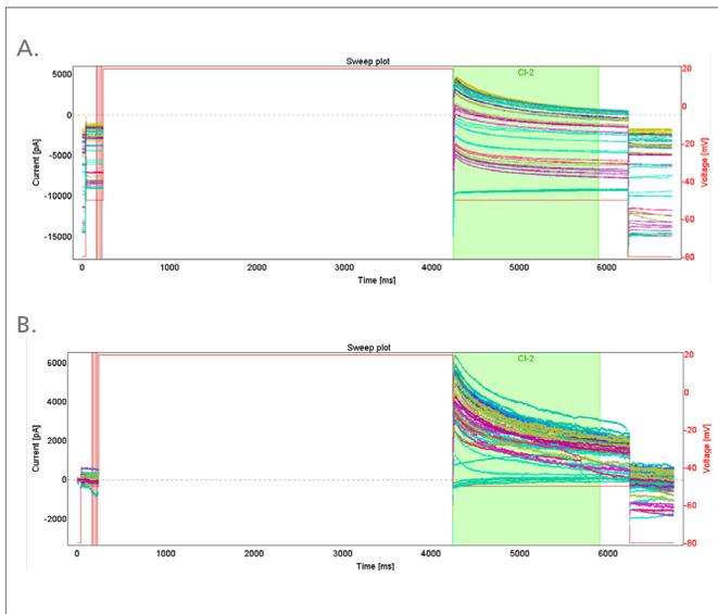
Fig. 2: Example of sweeps from a multi-hole experiment without (a) and with (b) online P/n leak subtraction.
