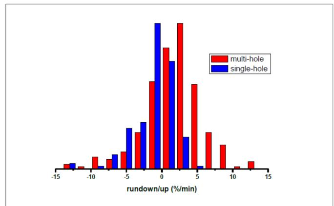
Fig. 8: Distribution of rundown rates in multi-hole and single-hole mode.
