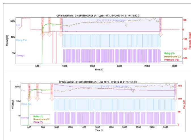
Fig. 1: Timelines from a representative well. By combining the two graphs, the total capacitance increases (red curve bottom plot) when whole-cell suction is applied (red curve top plot).
