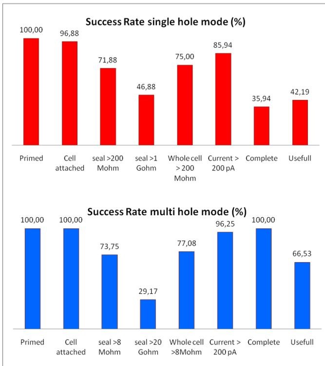
Fig. 5: Top: Success rate in single hole mode (n=64). Bottom: Success rate in multi-hole mode (n=240).
