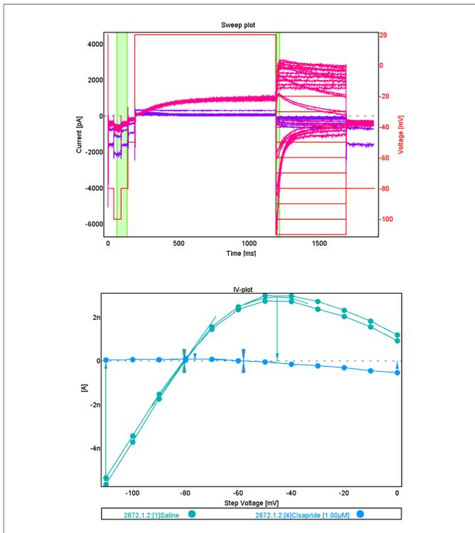
Fig. 9: The current-voltage relationship for determination of the reversal potential. Left: voltage protocol and raw current traces. Right: IV relationship, green line with physiological Ringer's solutions and blue line in the presence of 1  $\mu$ M Cisapride.
