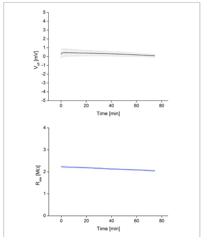
**Fig. 3:** Measurement stability of QPlate electrodes. The average voltage offset ( $V_{off}$ , top) and site resistance ( $R_{site}$ , bottom) were quantified in a cell-free assay and plotted as a function of time. Datapoints are average  $\pm$  SD between three QPlates (16 experiment sites per QPlate).
