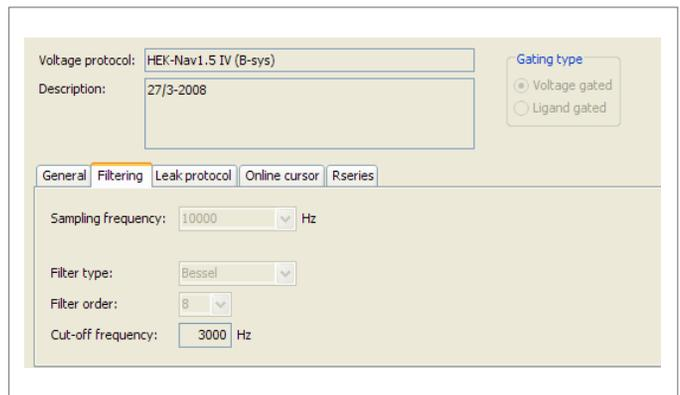
Fig. 7. Sampling frequency settings for CHO-Nav<sub>v</sub>1.5 experiments.
