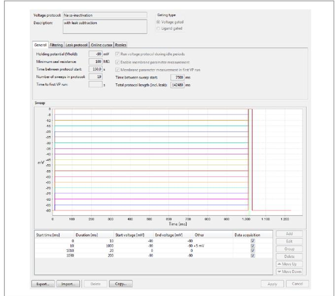
Data were sampled at a frequency of 10kHz (see figure 7). Rseries compensation was 100%.
