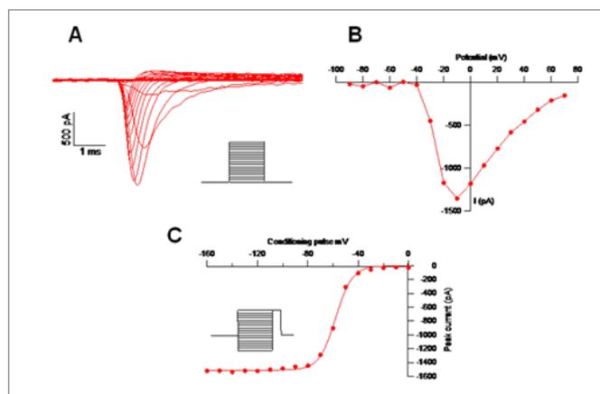
Fig. 1. A)  $\text{Na}^+$ -current in response to depolarizing steps; voltage protocol shown in the inset. B) I-V relationship of the  $\text{Na}^+$ -current shown in A). C) I-V relationship of the steady-state inactivation of the  $\text{Na}^+$ -channel. Voltage protocol shown in the inset.
