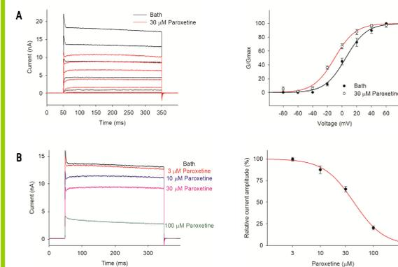
A) Cells expressing K<sub>v</sub>3.1a were voltage clamped from -80 to +60 mV for 300 ms in 20 mV increments. In the presence of 30 μM paroxetine, the voltage dependence of activation was shifted to more negative potentials: V<sub>0.5</sub>: 4.5 mV (control) to -10.08 mV (30 μM paroxetine).
