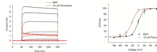
Cells expressing K<sub>v</sub>3.2 were voltage clamped from -80 to +60 mV for 200 ms in 20 mV increments. In the presence of 10 μM paroxetine, the voltage dependence of activation was shifted to more negative potentials: V<sub>0.5</sub>: -0.98 mV (Control) to -21.78 mV (10 μM paroxetine).
