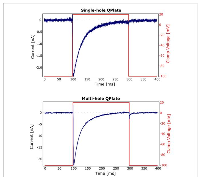
**Fig. 1:** Representative recordings of Ca<sup>2+</sup> current (blue) on a single-hole (top) and multi-hole (bottom) QPatch following a 200 ms depolarization from -100 mV to 20 mV (red) in Ca<sub>v</sub>1.2 expressing cells.
