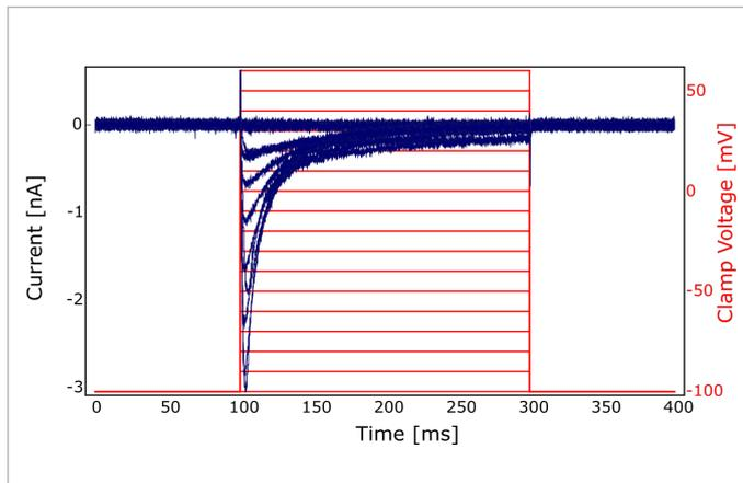
**Fig. 2:** Representative measurement of current-voltage relationship using a single-hole QPlate.  $\text{Ca}^{2+}$  current response of a cell expressing  $\text{Ca}_v1.2$  channels (blue) following a depolarization step protocol in  $10 \text{ mV}$  increments from  $-100 \text{ mV}$  to  $+60 \text{ mV}$  (red).
