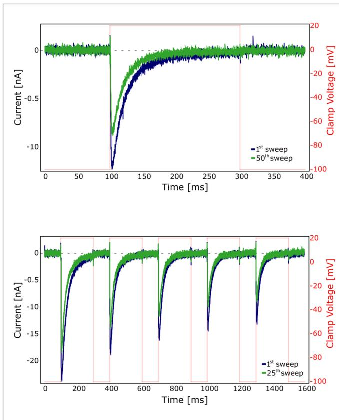
**Fig. 5:** Example current traces used for quantifying rundown. Top: 1<sup>st</sup> (blue) and 50<sup>th</sup> (green) depolarization in voltage protocol 2. Bottom: 1<sup>st</sup> (blue) and 25<sup>th</sup> (green) depolarization train in voltage protocol 3. Rundown was quantified for the first depolarization of the train.
