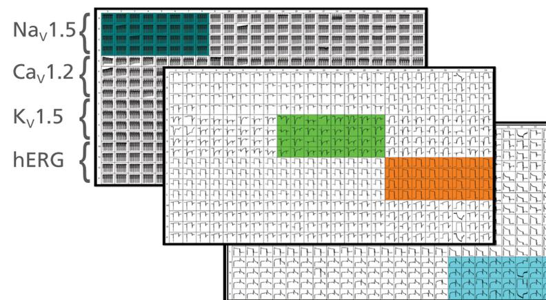
[Fig. 9]: Parallel measurement of 4 different cell lines.  $Na_v1.5$  (olive),  $Ca_v1.2$  (green),  $K_v1.5$  (orange) and hERG (cyan) were measured by applying the according voltage protocols. Quarters containing the matching intracellular and extracellular solution for the according ion channel are colored. The voltage protocol for  $Na_v1.5$  was followed by the identical  $Ca_v1.2/K_v1.5$  protocol and concluded with stimulating the hERG channel.
