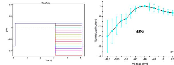
[Fig. 8]: IV protocol and normalized IV curve for hERG. Cells were depolarized for 3 s from -80 to +20 mV, followed by 2 s at a voltage between -120 mV and +20 mV in steps of 10 mV (left). The average peak tail current for each voltage step was normalized to the maximal response (right).
