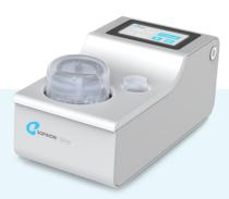
The centrifuge insert holds 1.5 mL lidless tubes (max spinning volume 1.0 mL) and operates at speeds up to 200 G. There's no maximum time limit, allowing flexible, ad hoc usage. The built-in magnetic stirrer ensures efficient cell stirring during processes.
