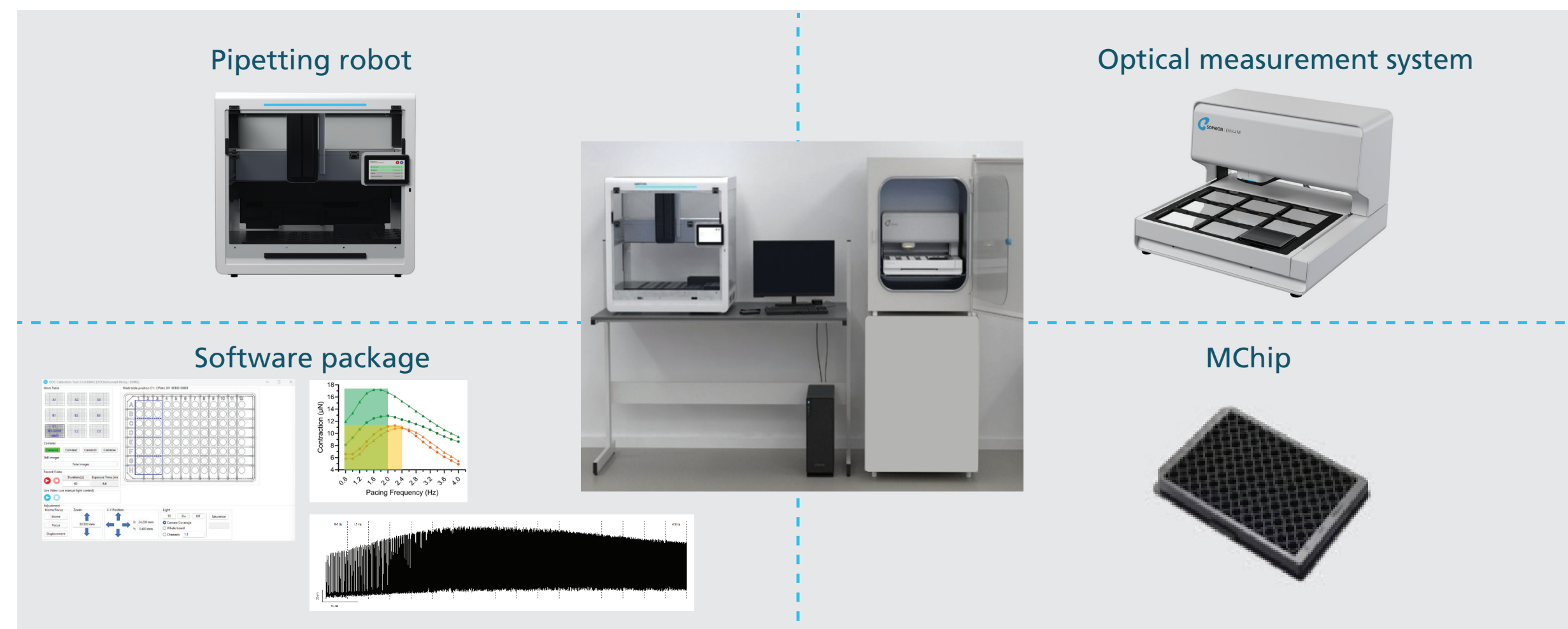
Fig. 1: Ethica M solution: The package includes: 1) An optical measurement system with high-speed camera and integrated pacing units, with slots for holding nine MChip consumables. The system is placed in a cell-culture incubator (not included with the system). 2) A 96-well plate format consumable, the MChip, has customizable mini-wells for casting contractile tissues and integrated pacing electrodes. 3) A pipetting robot is used for dispensing the cell/ gel matrix into the MChip for tissue formation. The pipetting robot has a HEPA filter and UV lamp for sterile handling of the pipetting process. 4) A user-friendly software package including an Assay scheduler, useful for long-term studies, to automatically tracks tissues and perform data acquisition and the Analyzer software that extracts key contractility parameters and presents results graphically or in an exportable format.
