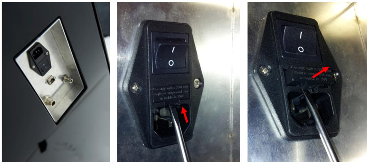
Figure 14 Left photo: Bulkhead plate placed on the rear right of Qube when looking at it from the rear side. The plate has the power inlet, main switch, Ethernet connection, and inlet for pressure and vacuum. Center and right photo: Arrows indicate how to open the main power input fuse compartment by placing a screwdriver in the slot under the compartment and pulling it out
