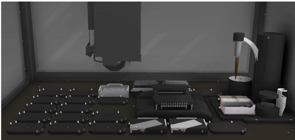
Figure 6 Qube worktable. The use of the available slot plates can be tailored depending on the assay. The mechanical layout may vary depending on the specific Qube configuration
