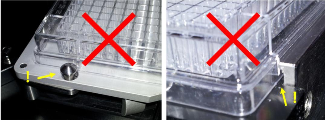
Figure 69 Example of an MTP with medium flange height in an active tip rack slot. The flange is too high to fit under the retainers and the MTP is therefore not compatible with the slot plate
