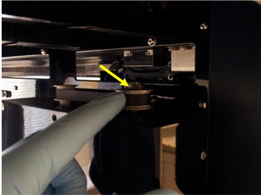
2. Move the 384-robot and thereby gripper arms fully out of the BCI by gently moving it by hand. Be careful to ensure that the gripper arms and potentially QChip 384 do not collide with any mechanical parts when moving the robot
