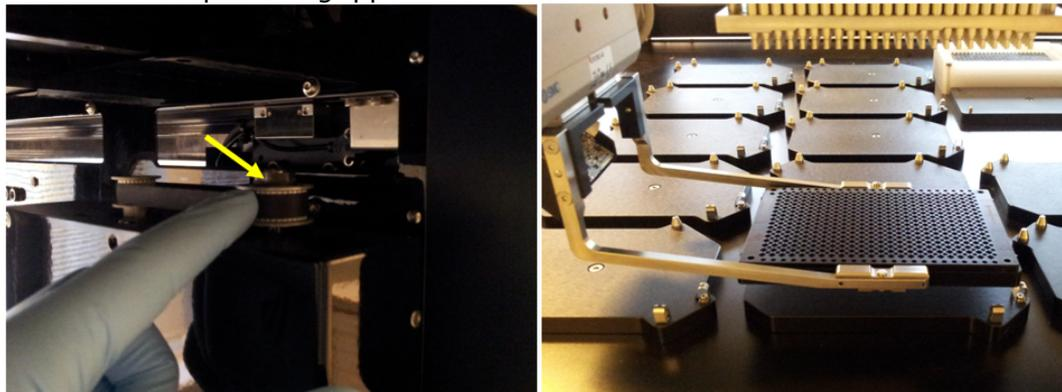
3. Use a flat tip screwdriver to turn the screw at the side of the gripper module in the clockwise direction. The gripper arms will now open and release the plate
