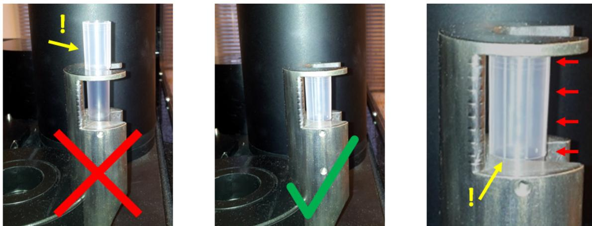
Figure 71 Placement of the ACP pipette tip in the tip ejector. Left: Incorrect position with the pipette tip resting on top of the ejector. Centre: Correct placement with the pipette tip collar inside the notch. Right: Close-up showing the collar pushed all the way to the back and is resting on the lower notch surface. The collar must not be squeezed into the lower part of the tool
