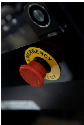
Figure 13 Emergency stop placed on the front in the right-hand side of Qube
