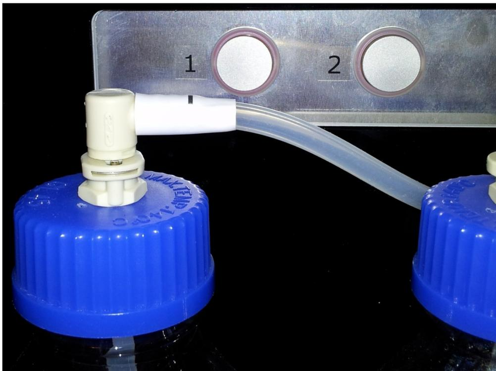
Figure 74 Photo showing two of the push buttons on the control and pump module placed behind the source bottles. The status LEDs light up the circumference of the buttons
