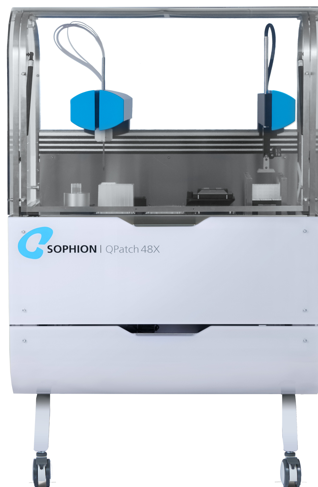
Fig. 1: QPatch II, the second generation of QPatch that carries out automated whole-cell voltage clamp recordings.
