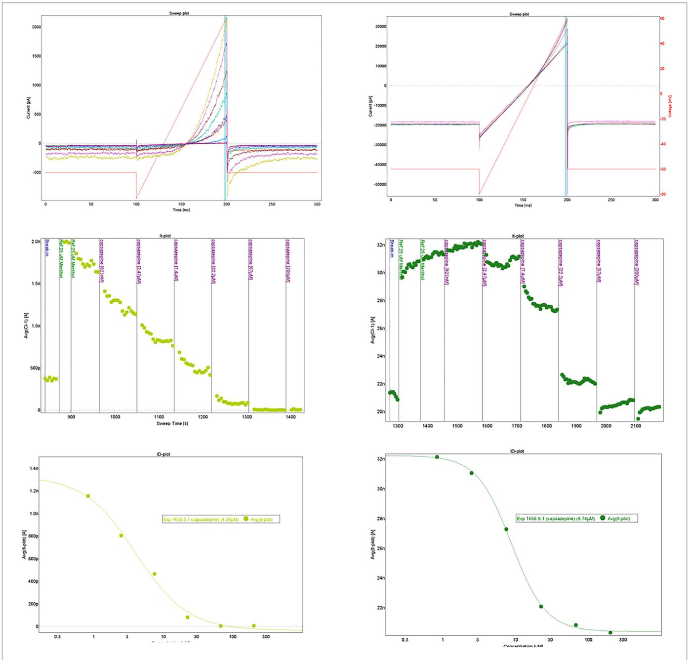
Fig. 16. Dose-response experiment with capsazepine tested in the presence of 25  $\mu\text{M}$   $\gamma$ -menthol. Left: Single-hole data in a dose-response experiment with capsazepine. Right: multi-hole data in a dose-response experiment with capsazepine. Top: raw data sweeps elicited with a ramp from -80 mV to +60 mV, middle: IT plot of current at +60 mV, bottom: Hill fit.
