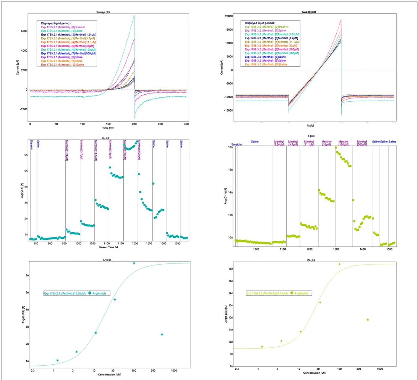
Fig. 15. Left: Single-hole data in a dose-response experiment with +/-menthol. Right: multi-hole data in a dose-response experiment with +/-menthol. Top: raw data sweeps elicited with a ramp from -80 mV to +60 mV, middle: IT plot of current at +60 mV, bottom: Hill fit.
