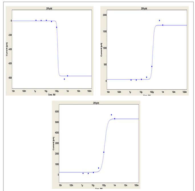
Fig. 7. Representative Hill fit of the concentration - response relationship to (-)-menthol. From the left: current level at -50 mV, +20 mV and +50 mV, respectively.
