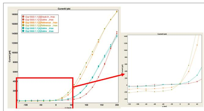
Fig. 1. Representative IV plot of TRPM8 response to saline and racemic menthol ('reference'). An enlargement of the response at negative potentials is shown to the right.
