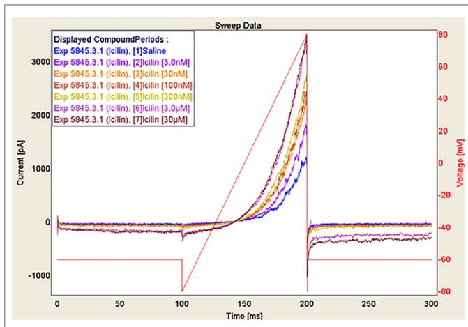
Fig. 9. Raw current traces of the response elicited by a voltage ramp from -80 to +80 mV, when subjected to increasing concentrations of icilin.
