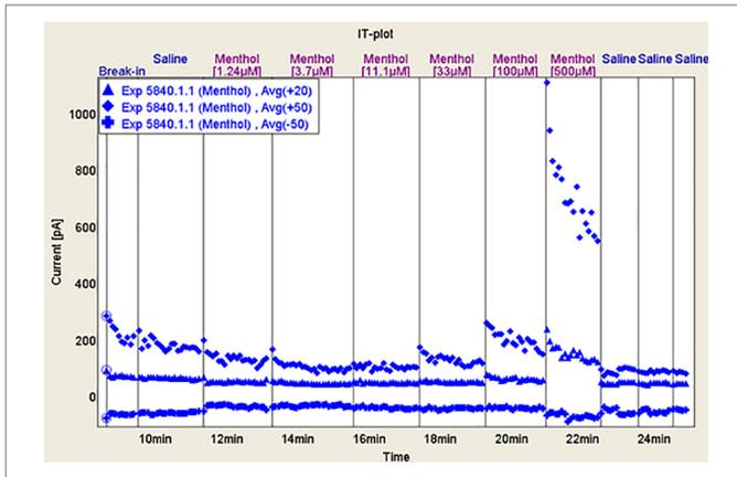
Fig. 3. Representative IT-plot of showing current values at +50 mV (◊), +20 mV (Δ) and -50 mV (+), in response to increasing concentrations of racemic menthol.
