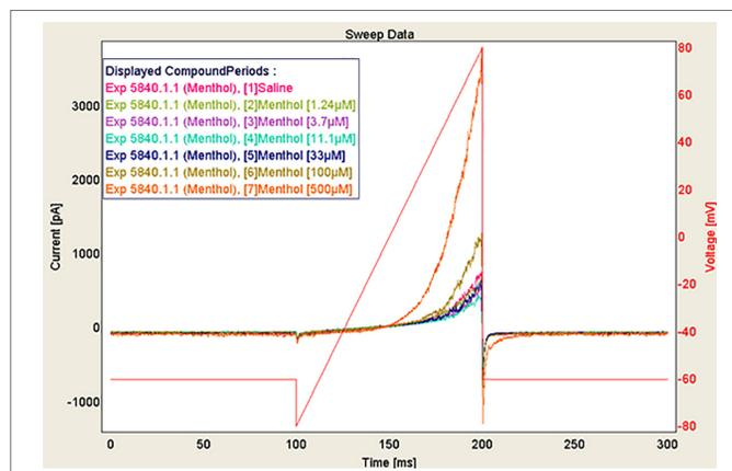
Fig. 2. Representative raw current traces of the response elicited by a voltage ramp from -80 to +80 mV, when subjected to increasing concentrations of racemic menthol as indicated.
