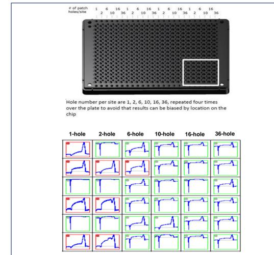
**Figure 2.** Nav1.5 and hERG currents recording with mixed cell lines using a QChip384 D with a variation of hole per well. The upper panel shows the assay development QChip384 D with hole numbers covering 1 to 36 per well. The lower panel shows example current traces in the lower right 36 wells of the QChip. Either hERG or Nav1.5 was seen in 1-hole well. hERG and Nav1.5 currents were seen in multiple hole wells
