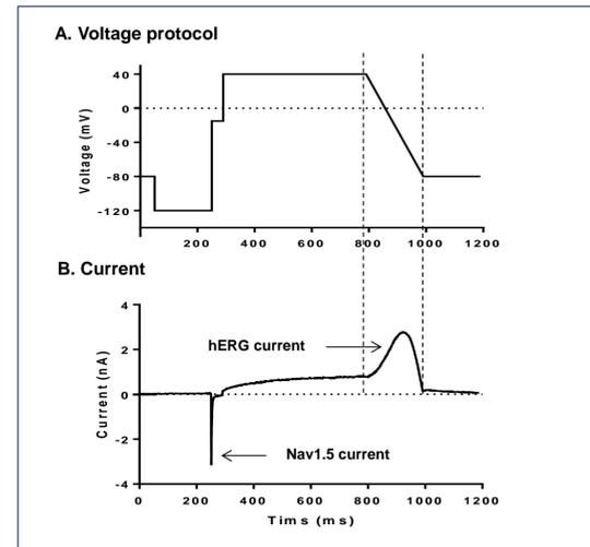
**Figure 1.** Temporal current separation based on discrete recording time windows with mixed cell lines using 10 hole QChip. (A) The voltage protocol for recording Nav1.5 and hERG currents. The step pulse from -120 mV to -15 mV was used to elicit the Nav1.5 current. The ramp from 40 mV to -80 mV was used to induce the hERG current. (B) An example of current trace with both Nav1.5 and hERG currents.
