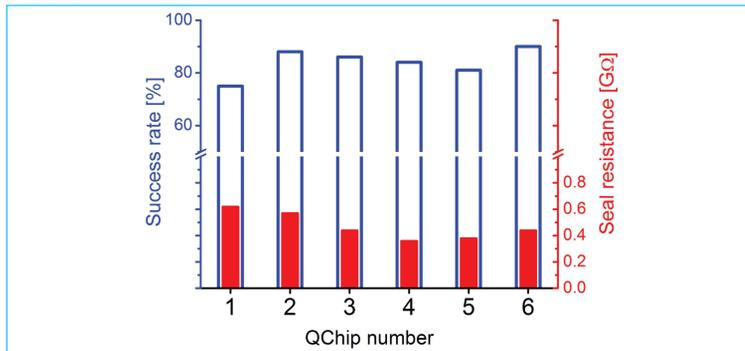
Fig. 1: Qube 384 TMEM16A assay performance: Overall success rates (blue) and whole-cell seal resistances (red) of 6 individual experiments (multi-hole QChips) performed on three different days. The filter criteria were defined as  $C \geq 5$  pF/cell;  $I_{\text{baseline}} \geq 0.5$  nA/cell and  $R_{\text{membrane}} \geq 0.1$  GΩ/cell.
