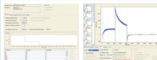
**Figure 1.** Graphical representation (red graph) of the hERG voltage protocol as viewed with the QPatch assay software (left). Typical hERG whole-cell currents (right). Ten single whole cell-current traces superimposed. Green cursors define time period in which the peak tail current is identified.
