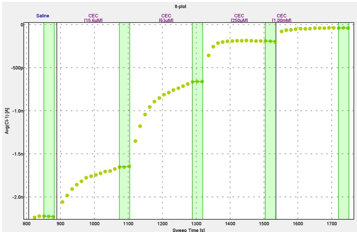
Fig. 5a. Time-current plot from a single cell with four increasing concentrations of CEC.
