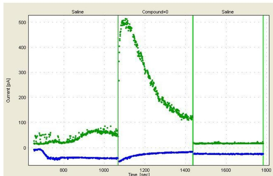
Figure 14. Green line is MIC measured at +95 mV and the blue is Icrac at -80 mV. The experiment type is passive depletion with EGTA followed by removal of extracellular Ca<sup>2+</sup> in the compound period which stops the Ca<sup>2+</sup> conductance of the CRAC channels but transiently stimulates MIC dramatically. There is no correlation between the two cursors.
